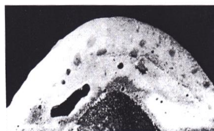
Figure 4. Section through the ceramic mass which was removed after sintering from the cylindrical cone casted from the non-noble (I.R.Scud și J.W.McLean)
