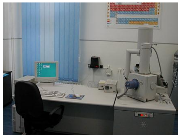
Figure 3. Phillips XL-30-ESEM electrono-microscope device, used for sample analysis.
